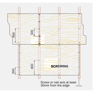
The length of the screws should allow the thread to overdrive the wing of the steel profile by around 5 mm. When using self-drilling tapping screws, the fixings on THEBAULT plywood panels should take place at least 10 mm away from their supported edges.
